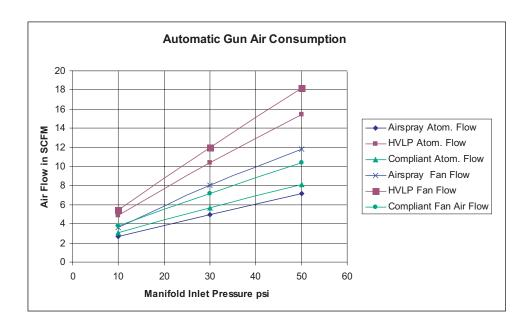
FIG. 2: Automatic Gun Air Consumption
